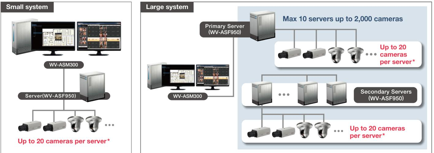
\*The WV-ASF950 includes license for 4 network cameras. To connect more than 5 cameras to the WV-ASF950, purchase WV-ASFE901 or WV-ASFE904 sold separately. When unregistered face detection function is selected, up to 10 cameras.
